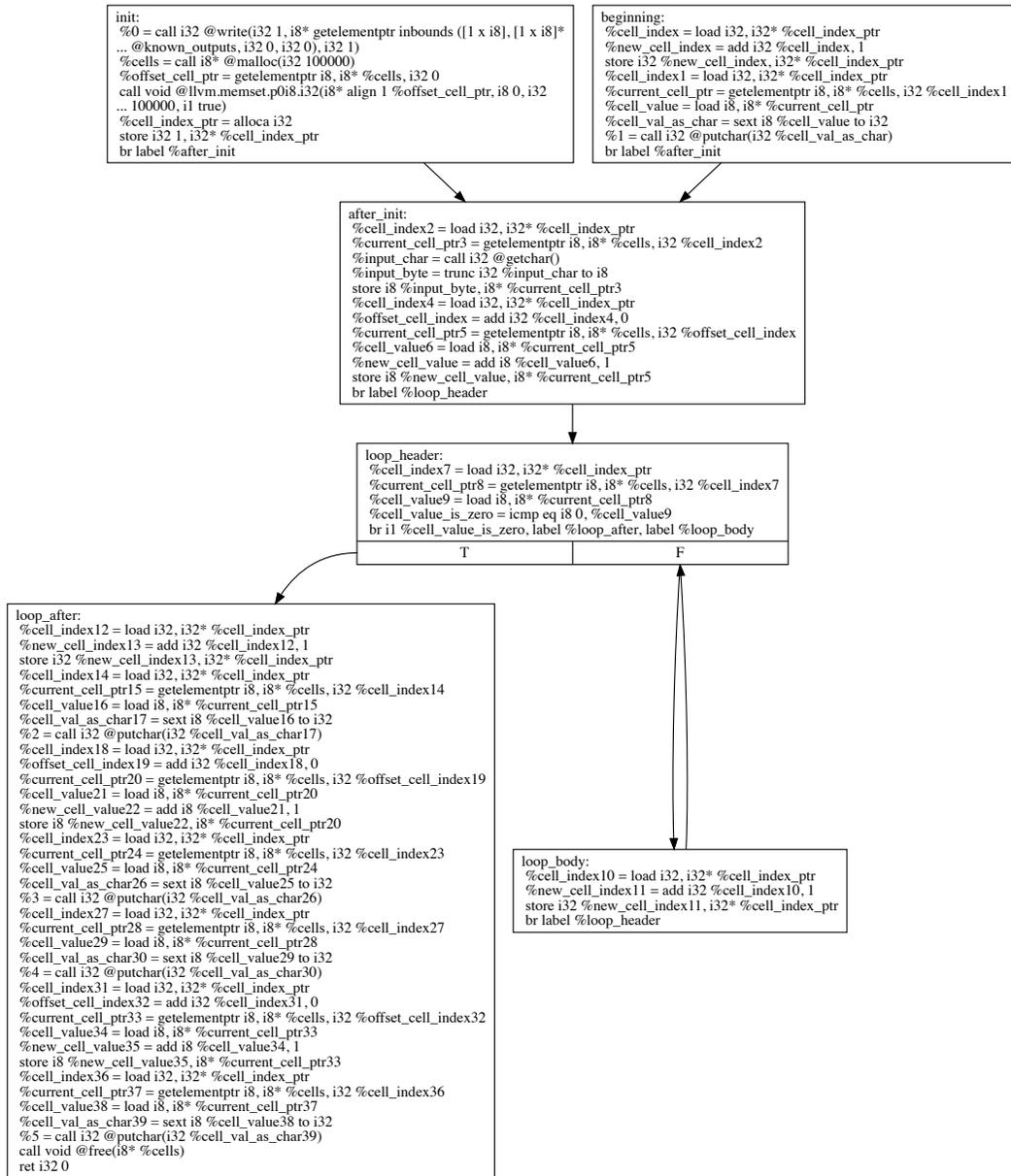
Figure 4.8. Control-flow graph of synthesized programs (2)
