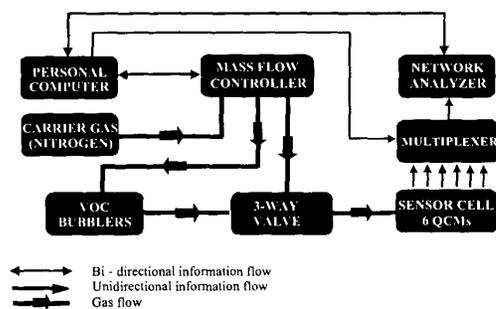
Fig. 1. Experimental setup for the Enose system.
