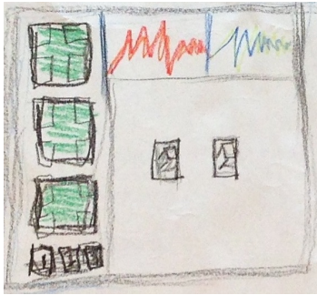
Figure 1: A distributed system design based on light switches. The line graphs at the top show the time series consumption of the room and the whole house. The green squares on the left allow the users to observe the consumption of the outlets in the room, as well as toggle them. Design by ST1.
