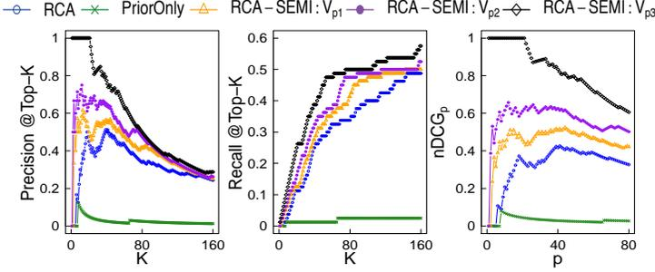
Fig. 9. Comparison on BIS data using prior knowledge. RCA-SEMI: $\mathcal{V}_{p1}$ , RCA-SEMI: $\mathcal{V}_{p2}$  and RCA-SEMI: $\mathcal{V}_{p3}$  refer to running RCA-SEMI with  $\mathcal{V}_{p1}$ ,  $\mathcal{V}_{p2}$  and  $\mathcal{V}_{p3}$ , respectively.
