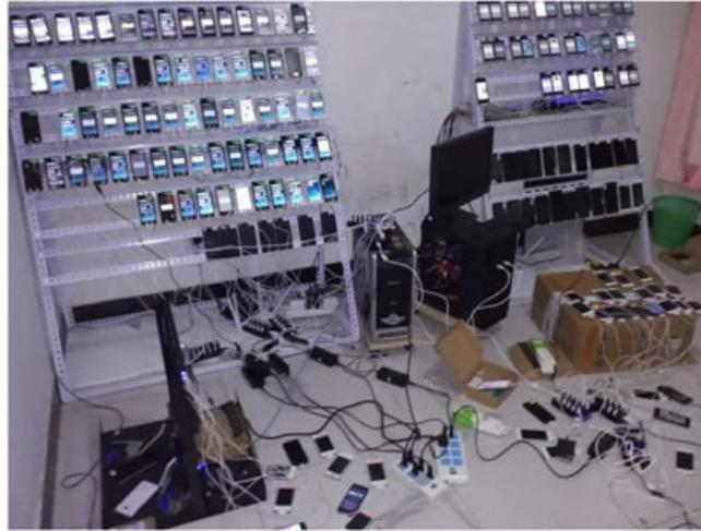
**FIGURE 1** Programmatically controlling massive iOS devices as a service (<http://shemeitong.com/index.php/anli/show/46.html>) [Colour figure can be viewed at [wileyonlinelibrary.com](http://wileyonlinelibrary.com)]
