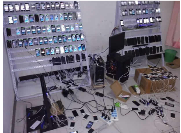
Figure 1: Programmatically controlling massive iOS devices as a service ( http://shemeitong.com/index.php/anli/show/46.html ).
