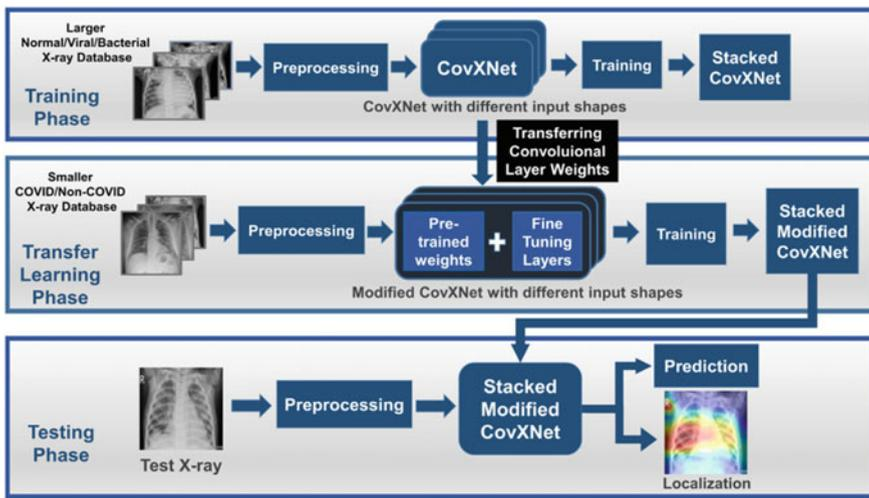
Fig. 15 The workflow of CovXNet [10]
