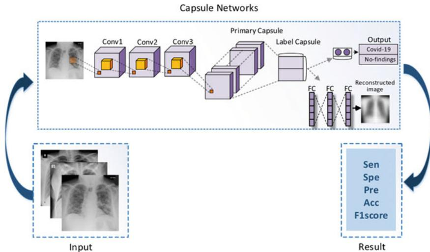
Fig. 20 Flowchart of the CapsNet [18]
