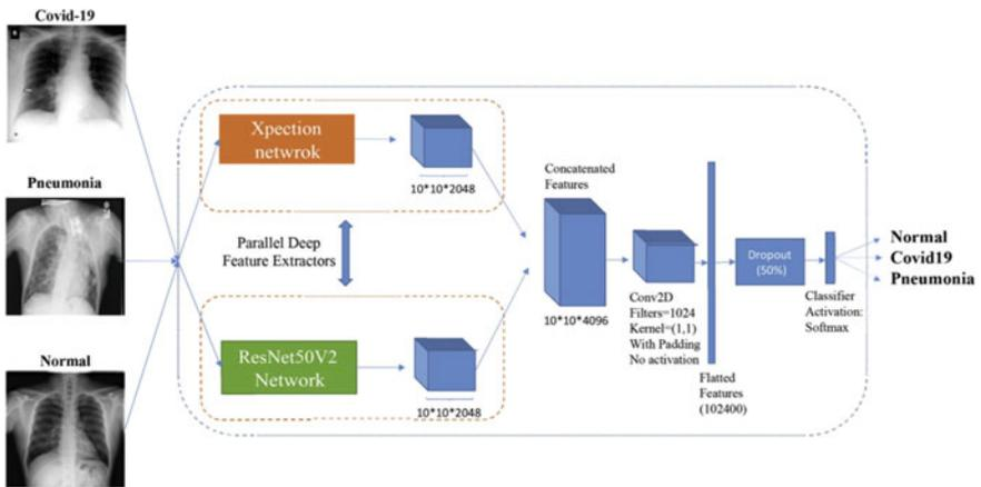
**Fig. 22** The architecture of the Hybrid Approach using Xception and ResNet50V2 [20]
